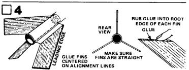
Rub glue into the root edge of each fin and allow to dry. Apply glue to the fins again and position fins on the alignment lines in
