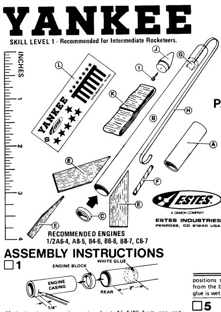
Mark the dummy engine casing (part A) 1/4" from one end. Spread a 1/2" wide band of glue around the inside of the body tube (part B) about 2" in from one end. Insert the engine block (part C) into this end. Push the engine block into place with the dummy engine casing until the mark on the casing is even with the end of the body tube. CAUTION: Once you have started to push the block forward, DO NOT STOP until it is in place, and then remove casing immediately!
