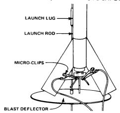
Slide launch rod through rocket launch lug and place rocket on launch pad. Make sure the rocket slides freely on the launch rod. Clean the micro-clips and attach them to the igniter wires. Arrange the clips so they do not touch each other or the metal blast deflector. Attach clips as close to protective tape on igniter as possible.
