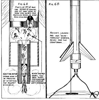
With this system it is necessary to allow an unobstructed path for the ignition gases from the igniter motor to the nozzles of the cluster. Only Series II
