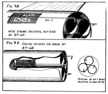
In the second system the engines are first glued or taped together, and then inserted into the rocket body. It is usually easier to obtain and maintain correct alignment by gluing the engines together than by taping them together. Enough tape is then wrapped around the outside of this group of engines to give a very tight
