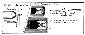
The loops of the coil must be spread far enough apart so there will be no possibility of one part touching another, even with the kleenex tamped in place. The parts of the nichrome leading to the coil must come out on opposite sides of the nozzle with the kleenex tamped in between them.
