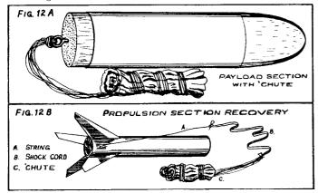
The best way to protect parachutes from the heat of the ejection charge is to use wadding and plenty of it. The wadding should be flameproofed. Flameproof cotton or flameproof tissue paper will work, but rock wool,
