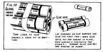
friction fit inside the rocket body. Finally, facial tissue or similar paper is tamped tightly into all holes around and between the engines to seal the rear of the rocket and control the ejection gases. (See fig. 11.)
