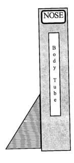
Using the fin marking guide provided, mark lines up and down the airfame to align the fins in the next step.
