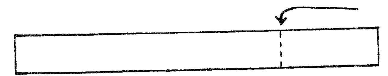
5. Cut two slots in the scrap of body tube 1/2" wide and 1.5" apart. Thread the shock cord through the mount and glue the assembly to the inside of the main tube. Be sure it is far enough down to allow the nose cone to slide on.
