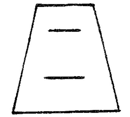
6. Glue the fins to the motor mount assembly 3/8" from the bottom. Glue them on one at a time and visually check for alignment from the back end. Set aside to dry, fillet all fins, let dry.
