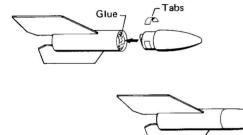
When each assembly is dry enough to handle, carefully slide the inside assembly into the outside assembly. Adjust fins to be neatly aligned, and carefully separate the assemblies.
