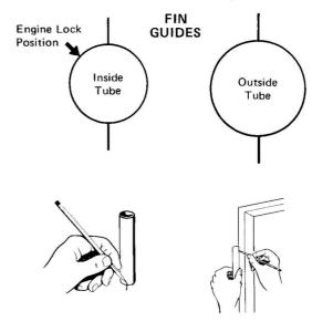
9 Apply glue to the indicated edges of two fins and position along lines drawn on the outside body tube. Remove, allow to dry, apply glue again, and re-position. Allow to dry standing vertically, and check alignment.
