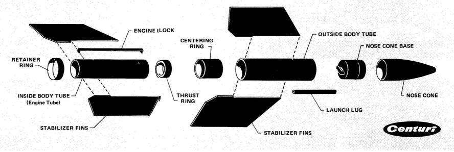
3 Run a bead of glue around the tube, above the pencil mark. Slide the retainer ring into place, 5/8" from the end. Apply a drop of glue where the engine lock sticks into the tube. Wipe away any excess glue, before it dries.
