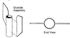
The remaining 2 fins are glued on the engine tube in a different manner. Use pre-gluing technique, as before, but leave the gaps between fins and tube. Allow to dry standing upside down, and check alignment as before.
