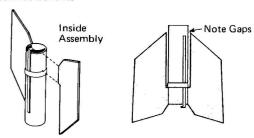
When the outside assembly is dry enough to handle, run a generous bead of glue around the inside aft end of the tube. Push the centering ring in place with a firm turning motion until it is recessed about 1/4".
