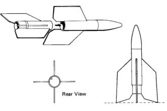
15 It is extremely important to strengthen the finbody tube joints because of the stresses received in flight and recovery.
