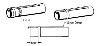
4 Carefully push the die-cut fins from their sheet. Start at one point on each fin and work gently around. Each fin is identical, but they are glued onto the body tubes differently. Study this diagram to understand their arrangement, before going to the next step.
