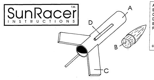
Body tube (ET-5) В Nose cone (BC-5) С Baisa (BAL10009) D Launch lug (LUG125) Template (TEM-10009) Ε Decal (D10009) Items E and F are not
