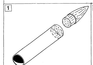
Apply glue to the inside of the body tube and glue the nose cone to the tube.
