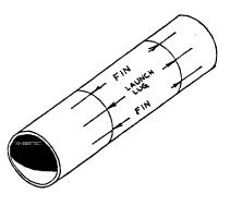
Cut out the fin placement template and wrap it around the tube. Use a pencil and mark the fin and launch lug locations.
