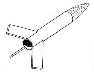
Glue on the fins with one at a time with white glue. Wait for each fin to dry before applying the next fin.
