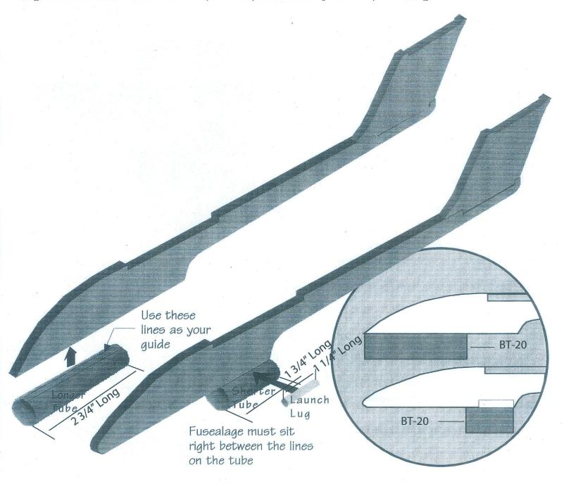
Once the glue is dry on those tubes, find the little white **launch lug**. Take the fuselage with the round nose and glue it into the "corner" between the motor tube and the fuselage. Make sure the back of the launch lug is at the very back of the tube. That will help the model slide smoothly later when you launch it.
