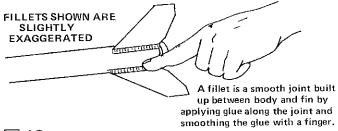
13 Apply a glue fillet to each fin joint. Holding the rocket horizontally, apply a line of glue to the joint and smooth it out with your finger. Support the rocket horizontally until the glue drys on all six fillets.
