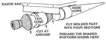
Using a razor saw or sharp knife, cut the molded nose cone/nozzle section into four parts as shown. Discard the two small conical sections previously attached to the nozzle. Lightly sand both front and rear edges of the nozzle section to remove any small plastic flash or burrs. This is best accomplished by rotating the part over fine sandpaper placed on a flat surface.
