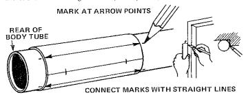
Qut out the marking guide from the pattern sheet (part D). Wrap it around one end of the body tube (part E). Mark the tube with a pencil at each arrow point at both ends of the marking guide. Remove the guide and draw straight lines connecting each matching front and rear marks. (The edge of desk drawer or a door frame makes a suitable guide for drawing the lines.) Extend the launch lug line the length of the tube.
