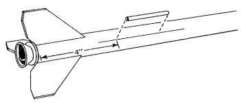
12 Glue the launch lug (part I) to the body tube on its line. The rear of the lug should be 4" from the rear of the body. Align it straight on the body.
