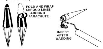
**T-13** Fold the parachute into a triangular shape. Roll 'chute tightly as shown and wrap shroud lines around it. If 'chute is too large, unroll it and repack until it slides easily into rocket. A fit that is too tight may prevent parachute from ejecting properly.
