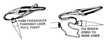
17 When all the paint on the nose cone and rocket body is dry, pass the parachute shroud lines through the loop on the nose cone. Pass the parachute through the shroud line loop ends and draw the lines tight against the nose cone loop. Set the knot with a drop of glue. Tie the free end of the shock cord to the nose cone.
