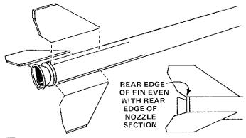
11 Glue the fins to the body tube on the fin alignment lines drawn in step 3. Refer to the illustration to be sure you position the fins correctly. Adjust the fins so they project straight away from the body tube. Do not set the rocket on its fins while the glue is wet.
