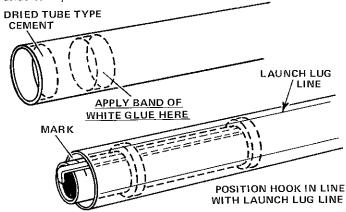
8 Test fit the engine mount assembly into the rear of the body tube. It should slide in easily. If not, sand the outside of the adapter rings until a smooth fit is achieved. Remove the engine mount and apply a band of white glue around the inside
