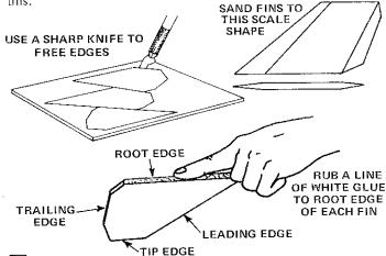
Fine sand the die-cut balsa sheet (part G), then carefully remove the fins from it. Free the edges with a sharp knife. For semi-scale appearance, sand the leading, trailing, and tip edges of the fins round. For full scale appearance, sand the fins as shown in the illustration. Leave the root edge of each fin square so that they can be properly glued to the body tube. Rub a line of white glue into the root edge of each fin and set aside to dry.
