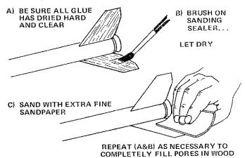
15 When all the glue on the outside of the model is dry, prepare the fins for painting. Apply at least two coats of sanding sealer to the fins. Let dry and sand lightly between coats. Do this until the tiny holes in the wood are filled and everything looks and feels smooth.
