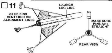
Rub glue into the root edge and dowel ends of each fin and allow to dry. Apply glue to the fins and dowels again and position fins on the alignment lines in positions shown. Adjust the fins so they project straight away from the body tube. DO NOT set the rocket on its fins while the glue is wet.
