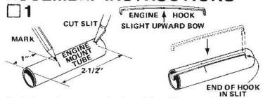
Mark the engine mount tube (part A) at 1" and 2-1/2" from one end. Cut a 1/8" long slit at the 2-1/2" mark. Gently bend the engine hook (part B) so that it bows upward very slightly in the middle. (Study the drawing — Don't bend the wrong way.) Insert one end of the engine hook into the slit in the tube.
