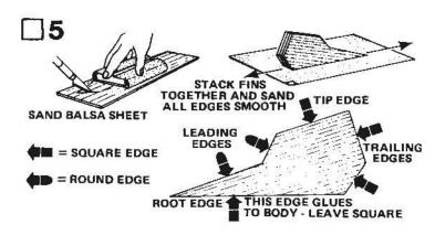
Fine-sand the balsa die-cut sheet (part E). Free the fin edges with a sharp knife, then carefully remove the die-cut fins from the sheet. Stack fins together as shown and sand all four sides as illustrated. Lightly sand both sides of each fin. Sand the leading edges of each fin to make them round. Leave the root (body) edge sanded "flat". The root edge may be identified by careful comparison with the drawings. Leave the tip and trailing edges square also.
