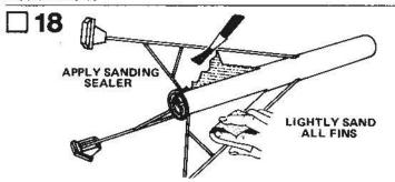
Proper application of sanding sealer makes the rocket look better and reduces drag so that the rocket will fly higher. However, this step is not essential to make a safe, attractive rocket. Apply a coat of sanding sealer to each fin. When sealer is dry, lightly sand all the sealed surfaces. Repeat sealing and sanding process until balsa grain is filled and smooth.
