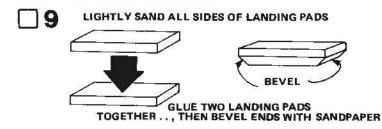
Use a piece of fine sandpaper to smooth the die-cut landing pads. There are a total of six. Glue the landing pads in pairs as shown to make 3 completed units. Use sandpaper to bevel two ends of each completed landing pad as shown.
