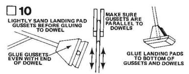
Lightly sand all edges of the 6 landing pad gussets. Be careful to keep all edges square. Glue the gussets to the ends of the 9" dowels as shown. The bottom of each gusset should be even with the end of the dowel. When the glue has dried, glue the landing pads to the ends of the gussets and dowel ends as illustrated. Check to be sure the pads are centered on the gussets and are on the same vertical line as the fins. Let the glue dry completely.
