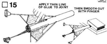
When the glue on the fin joints has dried, apply a glue reinforcement to each fin/body tube joint. Holding the model level, apply a line of glue to both sides of each fin joint and on both sides of the launch lug. Smooth out the glue with your finger. IMPORTANT — Support rocket on table edge as shown until the glue dries.
