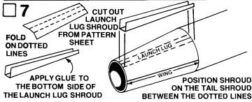
Cut out the launch lug shroud from the pattern sheet along the solid lines. Fold on dotted lines and apply glue to the bottom of the launch lug shroud as shown. Position the launch lug shroud between the dotted lines and even with the front and back of the tail shroud.
