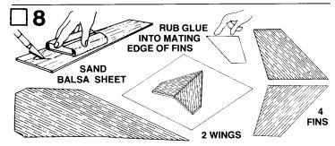
Fine-sand the balsa die-cut sheet (part G). Free the fin edges with a sharp knife, then carefully remove the die-cut fins from the sheet. Sort and identify parts as shown. Rub a line of glue into the mating edges of fins. Cover your work surface with waxed paper and apply a second bead of glue to the mating edges and press fin parts together as shown. Wipe away excess glue. Repeat assembly of the other fin parts and set aside to dry.
