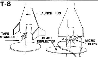
Slide launch rod through rocket launch lug and place rocket on launch pad. Make sure the rocket slides freely on the launch rod. Clean the micro-clips and attach them to the igniter wires. Arrange the clips so they do not touch each other or the metal blast deflector. Attach clips as close to protective tape on igniter as possible.
