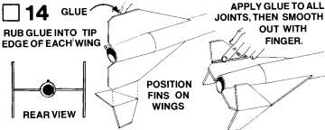
Rub glue into the tip edge of each wing and allow to dry. Apply glue to the wings again and center fins on wings as shown. Make sure fins and wings are square, then set aside to dry. When the glue on the fin joints has dried, apply a glue reinforcement to each fin/wing joint and to each wing/body tube joint. Smooth out the glue with your finger. Support rocket so rocket is level until the glue dries.
