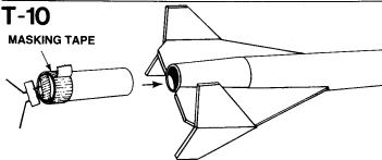
Wrap the rear of the engine with enough masking tape so that it makes a tight fit in the body tube. This fit must be tight to obtain proper parachute deployment. Insert the engine into the rocket so the rear of the engine projects 1/4" from the rear of the body tube.
