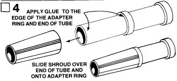
Apply glue to the edge of the adapter ring and the end of the tube. Slide the tail shroud into place so the small end is even with the end of the tube.
