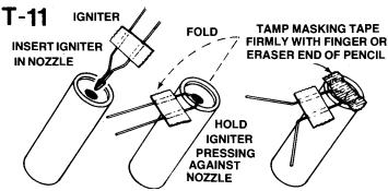
Select an engine and install an igniter as directed in the engine instructions. The engines recommended for use with this rocket are the A8-3, B4-4, B6-4, B8-5, and C6-5 made by Estes.
