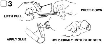
Cut out the tail shroud from the pattern sheet (part E) along solid black lines. Pre form the shroud by pulling it under a knife handle or pencil and up at the same time so it will curl up. Do this several times until the cone can be formed easily. Apply glue to the tab on the cone and position the edge of the shroud on the dotted line and press tab against inside of shroud. Hold it in place until glue sets.
