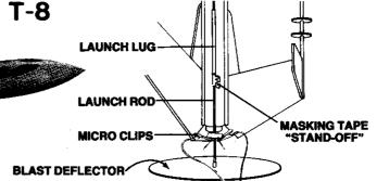
Slide the launch rod through rocket launch lug and place rocket on launch pad. Make sure the rocket slides freely on the launch rod. Clean the micro-clips and attach them to the igniter wires. Arrange the clips so they do not touch each other or the metal blast deflector. Attach clips as close to protective tape on igniter as possible.
