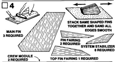
Fine-sand both sides of the balsa die-cut sheet (part E), then carefully remove the die-cut parts from the sheet by freeing the part edges with a sharp knife. Sand the edges of the fin parts slightly to remove any rough spots.
