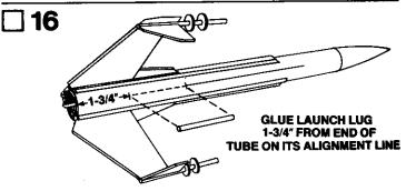
Glue launch lug (part N) to body tube on launch lug line. The rear of the launch lug should be 1-3/4" from the rear of the body tube. Align the launch lug straight along the tube.
