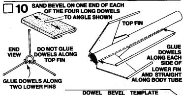
Locate the four 8-1/2" lengths of wood dowel from step 5. Sand a bevel on one end of each dowel to the angle shown. Glue the dowels, one on each side of the two lower fins, straight along the body tube. Do not glue dowels along the top fin.
