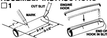
Mark the engine mount tube (part A) at 1", 2-1/4" and 2-1/2" from one end. Cut a 1/8" long slit at the 2-1/2" mark. Gently bend the engine hook (part B) so that it bows upward very slightly in the middle. (Study the drawing.—Don't bend the wrong way.) Insert one end of the engine hook into the slit in the tube.
