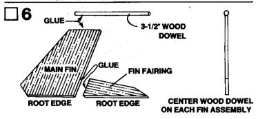
Assemble the fins as shown over a piece of waxed paper. Apply glue to edge of main fin and fin fairing as shown. Let glue partially dry. Apply second bead of glue to one edge and press parts together. Wipe away any excess glue. Repeat procedure for other two fin assemblies. Apply glue to a 3-1/2" dowel and position on top of each fin assembly as shown.
