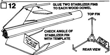
Cut out the stabilizer fin angle template from the pattern sheet. Apply glue to each stabilizer fin root edge and align two fins on each dowel as shown. Check angle of each stabilizer fin with template and allow glue to set. Do not set rocket on fins while glue is wet.
