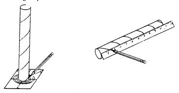
Mark the body tube for fin placement using the fin placement guide. Using a straight edge extend vertical lines up the body tube from the fin placement marks.
