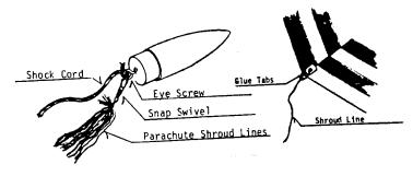
5. Put eyescrew in edge of nose cone. Attach the shock cord. The parachute is marked in inches. Cut with scissors to the desired size. For the Voyager, cut 14". Lay the parachute on a flat surface and attach shroud lines as shown. Punch a hole through the glue tab and tie the shroud lines to the parachute. Attach snap swivel. Repeat operation for second parachute.
