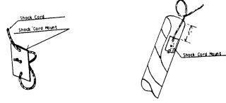
4. Install shock cord in shock cord mount as shown. Spread a heavy layer of glue over the side opposite the shock cord knot. Curve shock cord mount and insert into the nose cone end of the body tube and firmly press in place. Drawing shows the proper position in the body tube.
