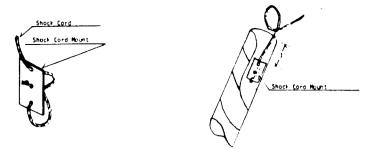
3. Install shock cord in shock mount as shown. Spread a heavy layer of glue over the side opposite the shock cord knot. Curve shock cord mount and insert into the nose cone end of the body tube and firmly press in place. Drawing shows the proper position in the body tube.
