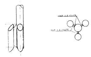
5. Apply a line of glue to the tip edge of the fairing and attach the stabilizer tube. Position as shown above. Stabilizer should be parallel to body tube. After dry apply glue fillets to attached points of stabilizers to fairings.
