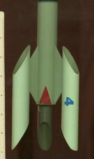
Nose Cone: 3.5" (from shoulder to tip) Fit BT55. (From BalsaMachining.com Shape=9, Size=5, Q=1.325, L=3.5, M=.75, I=1.283, A=1.0) Body Tube: 18" length. Use BT55. Fin Material: 1/16" Plywood Stabilizer Tubes: 5.5" length. Use .908 BT from Totally Tubular. Engine Mount Tube: For 18mm, Use BT20, 3" long For 24mm, Use BT50, 3" long Thrust Ring: For BT20 or BT50 Centering Rings: Use CR20-55 or CR50-55 Shock Cord: At least 36" length Parachute: 18" Launch Lug: 1/8" X 1"
