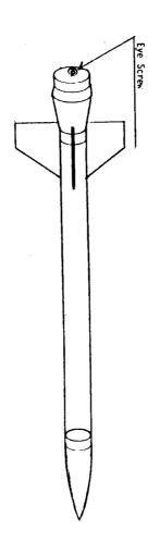
After the fins are dry glue the transition section in the end of the the transition. A small amount of glue may be used to keep the eyeupper body tube as shown. Now twist the eyescrew into the center of screw from coming loose. Attach the nose cone.
