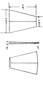
Sanding the fins for the booster section: If you are building your body tube. model to scale sand and shape fins as shown in the detailed drawing. For sport flying you may want to simply round the edges of the fins. If so round all edges except the red one. The red edge attaches to
