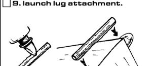
Once the fuselage and wing assembly is thoroughly dry, apply a generous bead of glue to the launch lug.
