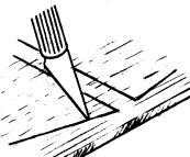
Cut fins from fin sheet. If possible use a ruler to help you get a good straight edge. Large fins are for the booster and small fins for the body
