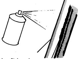
For best flight performance and appearance your rocket should have a smooth, hard finish. The cardboard and balsa parts should have several coats of sealer, sanding lightly between each coat. When painting, if a brush is used, sand carefully after each coat. If a spray can is used, apply several light coats avoiding runs. Bright colors are best for easy spotting and recovery.
