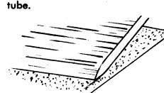
Sand the three edges of fins that do not attach to body tube. Sand the fin surfaces smooth.
