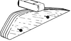
Cut a notch down the middle of the stabilizer fins, on the side opposite
