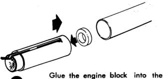
engine compartment so that it is flush with the end, and let dry. Put some glue on your finger, and spread it around up inside the 12" body tube. Insert the engine compartment, by pushing hard until the end without the block is flush with the bottom of body tube. The use of the engine in the compartment will keep the tubes from being crushed. If you have to use a new engine, be sure to wipe all the glue off.
