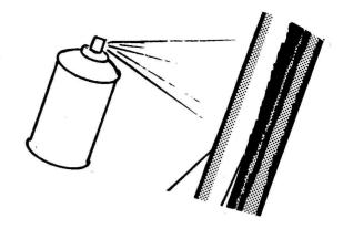
For best flight performance and appearance your rocket should have a smooth, hard finish. The cardboard and balsa parts should have several coats of sealer, sanding lightly between each coat. When painting, if a brush is used, sand carefully after each coat. If a spray can is used, apply several light coats to avoid runs. Bright colors are best for easy spotting and recovery.
