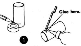
Place an engine block against engine compartment, and mark with a pencil as shown. Apply glue inside this end of engine compartment, and insert engine block. Cut slit on the pencil mark, and insert engine clip.
