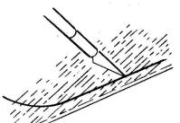
Cut glider fins from balsa fin sheet, pin together, and sand as shown in step 3. Cut ELEVON from wing.
