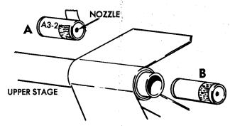
Once the upper stage engine is in place, slide the booster stage over the upper stage engine compartment (C). Wrap a layer of masking tape around the nozzle end of the B6-0 engine (D). Insert engine into booster stage, check for a tight fit, and add additional tape if needed (E). Make sure the B6-0
