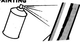
For best flight performance, and appearance, your rocket should have a smooth, hard finish. The cardboard should have several coats of sealer, sanding lightly between each coat. When painting, if a brush is used, sand carefully after each coat. If a spray can is used, apply several light coats avoiding runs.
