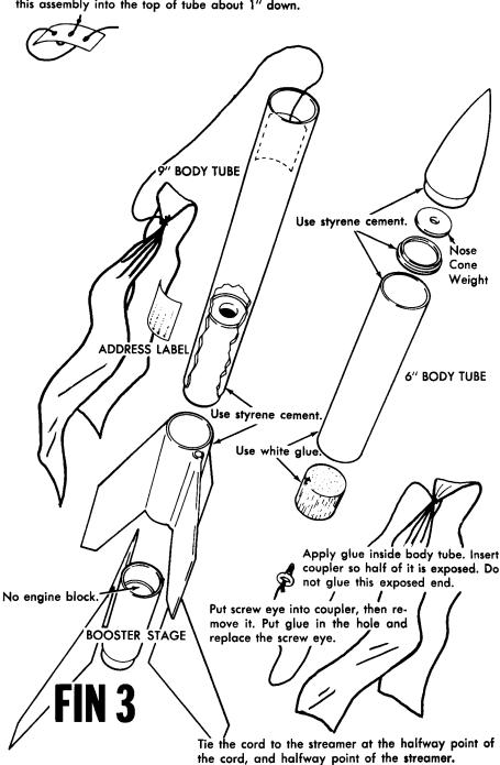
NOTE: If the balsa coupler is too large, sand the surface until a smooth fit is attained. In some cases the coupler may be loose. If so, wrap tape around the coupler until a good fit is achieved.
