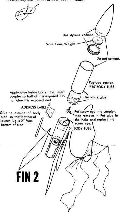
Tie the cord to the streamer at the halfway point of the cord, and halfway point of the streamer.
