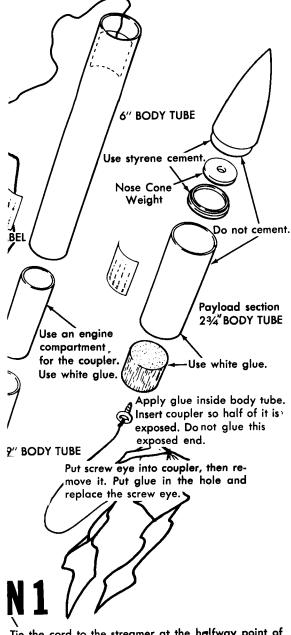
Tie the cord to the streamer at the halfway point of the cord, and halfway point of the streamer.
