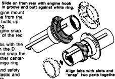
If D engine mount plate fits too tight - sand inside edges to loosen fit
