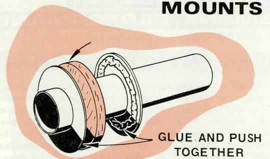
John Pauletich of Pueblo, Colo., suggests using a paper centering ring as a template to make a balsa centering ring. This gives extra gluing surface and strength to engine tube mountings in large body tubes.
