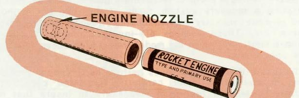
Larry DiGioia, Pittsburgh, Pa. and Lee Allen of Williamsport, Ind. are two of many rocketeers who have suggested a use for expended "D" engine casings. Use a sharp knife to clean out the casing and slightly enlarge the nozzle for ejection gases, thus converting your "D" engine casing to an adapter for launching a "D" bird with B or C engines.
