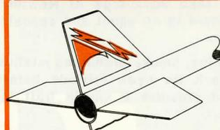
For easy to make paint designs, Bruce Burger of Syosset, N.Y., uses PRM-1 reinforcing paper cut to wanted design, applied to model, and then painted and removed.
