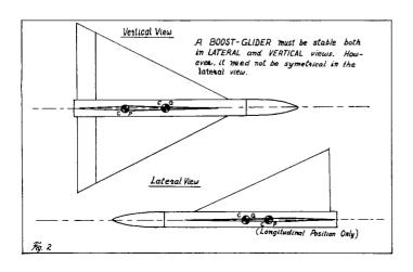
rocket stability is one in which very little corrective moment is applied because the rocket flies with little oscillation directly into the relative wind. While the air hitting the surfaces at an angle produces a component of force acting perpendicular to the body to push the rocket back into parallel with the relative wind, it also produces a component of force pointing directly rearward from the rocket, and parallel to the relative wind. This latter force is drag, and
