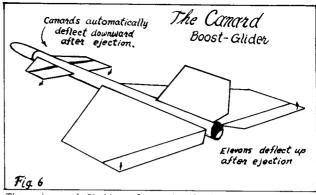
There is no definite rule as to the best aspect ratio for delta or flying wing designs. It seems that high aspect ratio wings give faster response to thermal currents than low aspect ratio wings. Low aspect ratio wings are slower to recover from dives. However, structural considerations also come into the picture, as we shall see in Part III.
