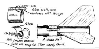
808 FIINT, Shawnee Mission, Kansas suggests a clean and easy way to hold a rocket off the wiring during countdown, if the fins do not hold rockets-end off of the launch-pad.
