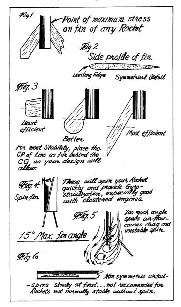
the point where the leading edge comes into contact with the body tube. A weak hold in this area may result in loss of the fin. (See figure 1.)
