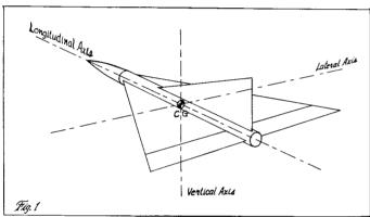
stabilized by locating the center of pressure behind the center of gravity in the manner detailed in Technical Report TR-1. This is going to have an obvious effect on the boostglider: Its wings must be located so that they bring the CP of the top view behind the CG by a substantial margin, and also its directional stabilizing surface, the rudder(s), must be located so that it brings the CP behind the CG in the side view.
