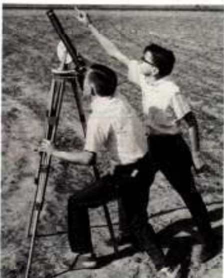
Two men are needed at each tracking station. One man operates the tracking device while the other aids in following the "track" and handles communications with the launch site.
