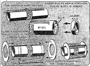
If this assembly in turn goes into a larger body tube, the adapter system must be extra strong. For a BT-55 size rocket the AR-5055 rings should be used. In larger tube sizes the rings should be reinforced with gussets as shown. Always use plenty of glue and let it dry completely.
