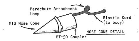
Attach an 18 inch plastic chute to the nose. It will fit easily, as well as larger 1/2 mil mylar chutes, if desired. A good idea would be to reinforce the chute by running the shroud lines over the top of the chute and attaching the lines with adhesive mylar. This will prevent the shroud lines from popping off.
