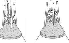
□ 16. Apply a thin ring of glue to the ring surface on the upper V-strut assembly. Also apply a small bead of glue to each of the upper joints. Slide the assembly into place as
