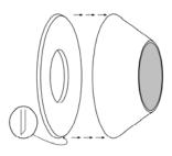
the rings off the edge. Sand a bevel on the edge to match the inside wall of the shroud. Remove the center circle and fit the ring over the bottom of the nose cone. Make sure the bevel side matches the inside of the shroud.
