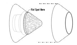
**5.** Punch out the large ring from the laser-cut sheet. The outside edge is cut partially through on one side with two laser cuts. Use your thumb to peel
