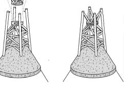
□ 17. Punch out the center hole in the upper jig. Center the base of the escape motor tail cone in the hole. Press it into place until the jig surface is flat with the bottom of the tail cone. Using a sharp pencil, mark the tail cone through the four holes. Remove and discard the jig. Apply a small dab of glue to each pencil mark and fit the escape tower into place. Check the assembly for alignment and set it aside to dry completely.
