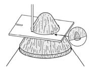
□ 15. Set the capsule and tower assembly vertically on a flat surface. Apply a drop of glue on the bottom joint of each leg of the lower V-strut. Slide the assembly into place using a slight turn to align the legs as shown. Use a small toothpick or sliver of wood to put small fillets at
