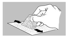
4. Round each leading edge and trailing edge of the main fins and the ends of the pod fins. Leave all the tip and root edges flat.
