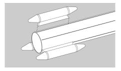
13. Apply glue to one of the main fins and position it along one of the remaining lines. Remove it, allow it to almost dry, reapply glue and reposition it. Allow this fin to dry before proceeding, checking for perpendicular positioning with the main body tube. Repeat for the other two fins.
