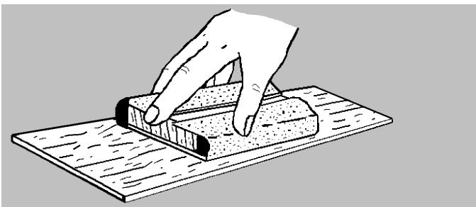
**3.** Carefully remove the laser-cut fins from the balsa fin sheet. Stack the fins together and sand off the holding tabs as shown in the illustration below. Remove the pod mounts and balsa strips and sand them in groups as you did the fins. The balsa strips will require some additional sanding later.
