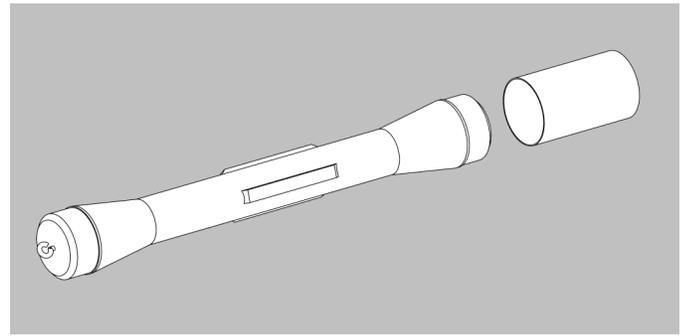
❑ **24.** Glue the nosecone to the top of the payload tube.
