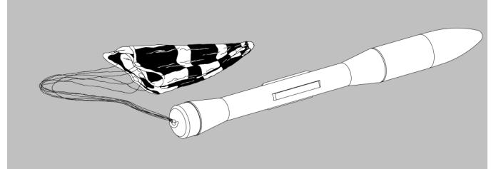
**26.** Prepare the shock cord as follows. Line up one end of the elastic shock cord with the free end of the Kevlar cord extending from the top of the body tube. Tie an overhand knot at the end of the two cords. Pull the knot tight and place a small drop of white glue on the knot to prevent it from loosening. Tie the loose end of the elastic to the screw eye on the payload section.
