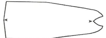
**# 14:** Test fit the top body wrap by pressing it into place on the plane. The "front" arrow between the two points of the body wrap should touch the mark you just drew. The rear should line up with the end of the body tube. Gently curl the body wrap so that it fits the contours of the model.
