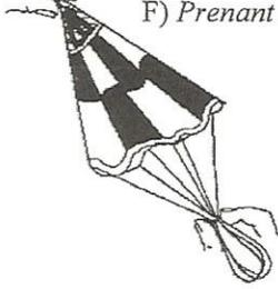
G) Pass parachute through loop and pull tight.
