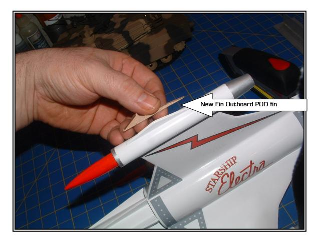
11- Make a mark ¼ inch aft of the forward most edge of the body tube. Glue the three forward fins with the leading point of each fin resting on this mark. These will be in alignment with the main fins. See next photo for clarification. You may want to use some tape to hold them in place while they dry. Go back and check all joints and add another coat of glue where needed. Let dry.
