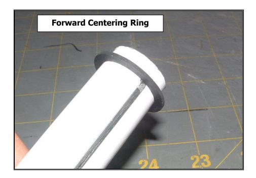
4- Coat the engine hook area of the engine tube with glue and slide the 2 inch engine retainer sleeve into place so that it butts up against the forward centering ring. See photo.
