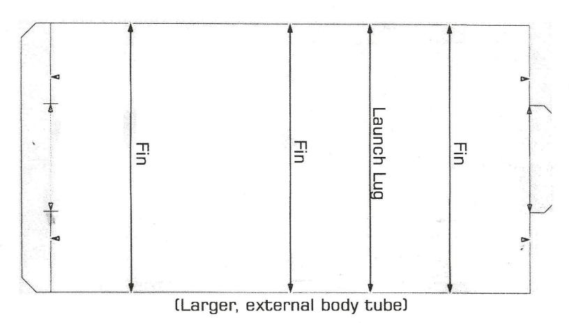
Main internal and external body tube fin wrap guide
