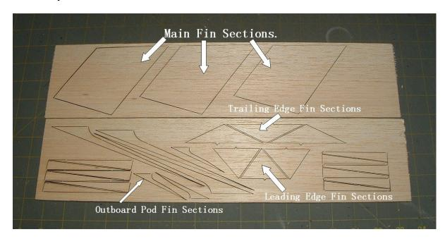
3- Note the layout of the pieces below. Pay particular attention to the direction of the wood grain and the *orientation tabs* (which can be sanded off later) as noted in the photos.
