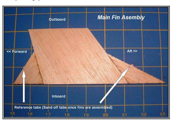
5- When the main fin assemblies have dried, carefully remove them and stack them together. Check to insure root edges are straight and consistent with all three. Sand and round the leading and training edges. Sand any excess glue from seams and fill any pin holes as necessary. Once the fins are attached, it will be difficult to do any heavy sanding so do as much finish work as possible at this point.
