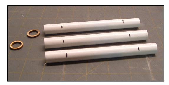
2- Glue a small pod tube ring at each of these marks. There should be exactly 1 inch between the end of each tube and each ring. Do this at each end of each of the three tubes.
