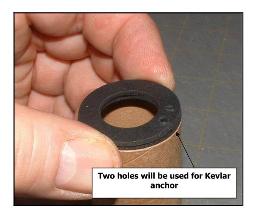
5- Pass the Kevlar thread through the two holes and tie off together so that it forms a loop. The knot should be on the opposite end from the rings. I use a square knot and then put one very small dab of thin CA glue to hold the knot. Test it to make sure it won't slip.
