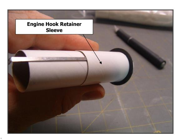
4- Glue the aft centering ring into place as shown. You may want to make a small notch on the inside of this ring to help it slide over the engine hook. Make sure the ring rests up against the engine hook retainer sleeve you installed in the last step. Let this assembly dry.
