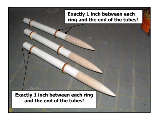
3- Locate the three LARGE pod tubes. Glue them in place over the smaller pod tubes so that the aft ring is even with the end of the larger tube as shown in the photo below. Do this with all three tubes. This will leave a space around nose cone on the front.
