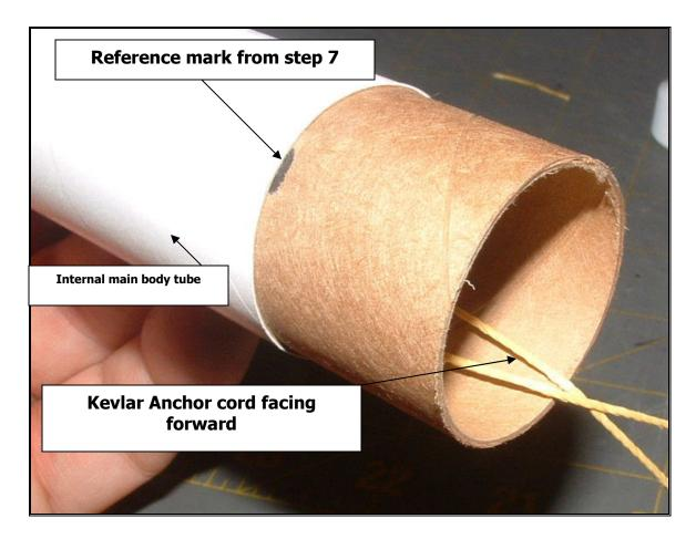
8- When the coupler has had a chance to dry, tie the shock cord to the Kevlar cord. Some modelers feel that putting a dab of glue on the elastic shock cord knot may make it brittle over time. I use a small drop of yellow glue when it involves this type of knot. If you choose to do the same, use the glue sparingly.
