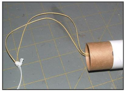
9- Now, thread the shock cord back through the opposite end of the tube. (You can pull it back through after the tube sections are joined) This will eventually be where the motor mount is installed but we'll do that a little later.
