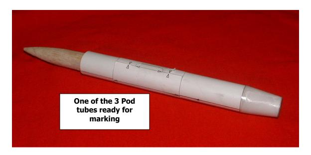
4- Using whatever method you are used to; connect all of your marks by drawing them the <u>entire</u> length of <u>each and every</u> tube. You should end up with five tubes, with alignment marks that go from one end of each tube to the other. The smaller internal body tube assembly should have six lines, the large external body tube 4 lines (one is a launch lug line) and the small pod tubes should all have two lines each.
