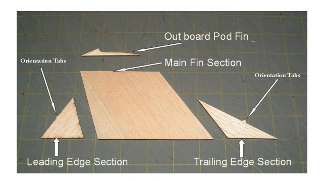
4- Using a piece of wax paper or saran wrap, pin down and glue the main fin pieces together. Use the root edge as a base line. I use a straight edge to keep the root edge straight. Observe the orientation tabs on the forward and aft pieces. These should help you orient each of these to the main piece. Once the assembly is dry, you can sand off these forward and aft tabs. The root edge is the edge that gets glued to the body tube or the pod tube. Make three sets. Let dry thoroughly.
